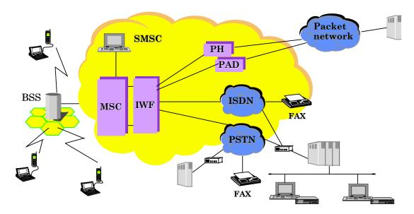
The IWF (Interworking Function) allows communicating with any "data network"
