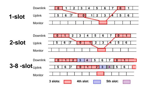
The figure suggests that the same slots are used in a regular interval. **This is not the case!** They are dynamically assigned to different MS!!!
